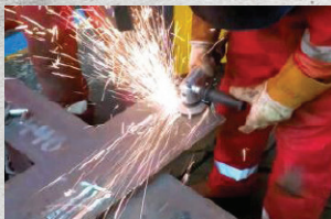
Ship Deck Paint Removal
